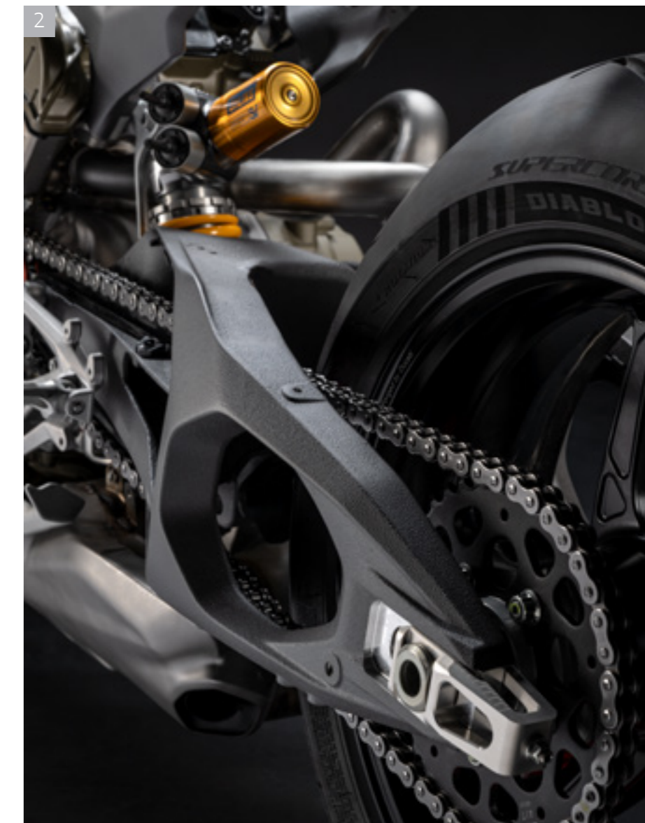
2 Fully adjustable Öhlins TTX36 (SV) S-EC 3.0 unit. Electronic compression and rebound damping adjustment with Öhlins Smart EC 3.0 event-based mode. Aluminium Hollow Symmetrical Swingarm
